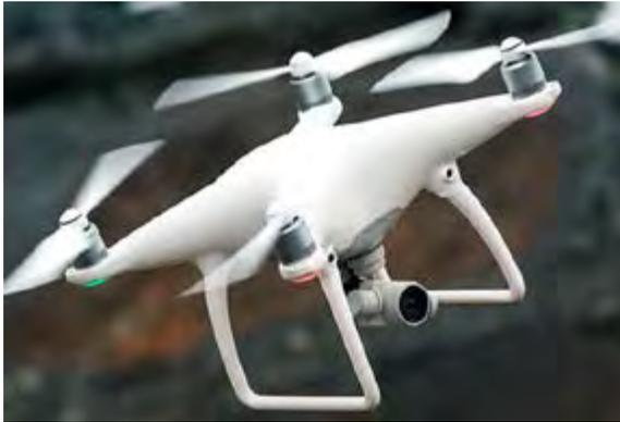
*The DJI Phantom 4 quad-copter drone, capable of flying programmed flight paths using GPS capturing high resolution aerial imagery to track changing land conditions over USAREUR Training Areas.*
